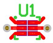
Figure 10. SiT1811 Layout example for board without bypass capacitor
