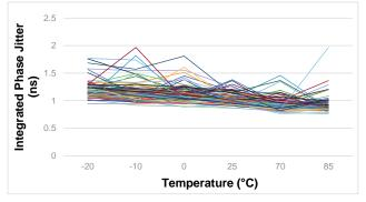
Figure 5. Integrated Phase Jitter, no supply noise over temperature for VDD = 1.5 V
