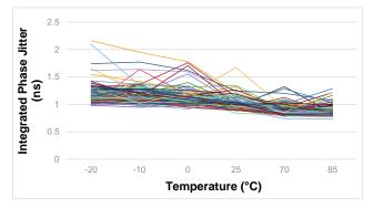
Figure 6. Integrated Phase Jitter, no supply noise over temperature for VDD = 1.8 V
