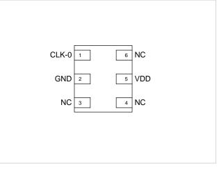
Figure 2. Pin Assignments (Top view) (Refer to Table 4 for Pin Descriptions)
