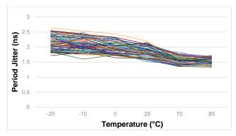
Figure 4. Period Jitter, no supply noise over temperature for VDD = 1.8 V
