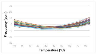
Figure 9. Frequency Vs Temp Stability
