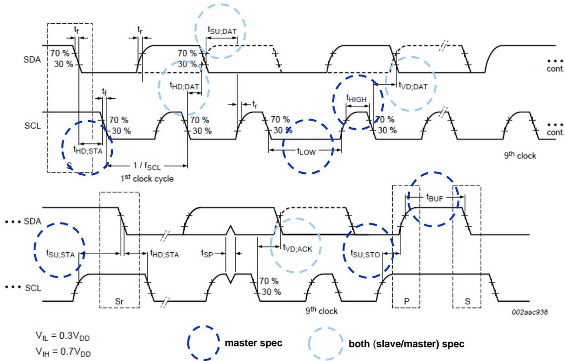
**Figure 34. I<sup>2</sup>C Timing Diagram**
