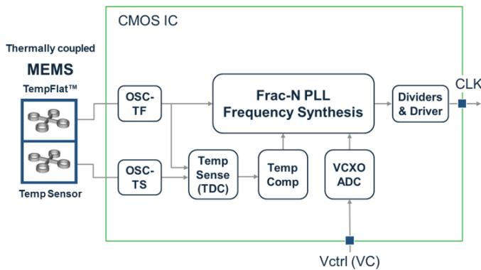
**Figure 23. Block Diagram – VCTCXO**
