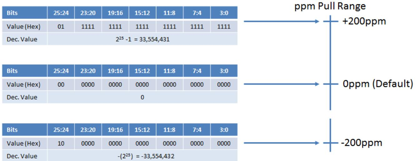
Figure 28. Pull Range and Frequency Control Word
