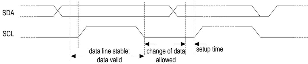
**Figure 29. Data and clock timing relation in I<sup>2</sup>C bus**
