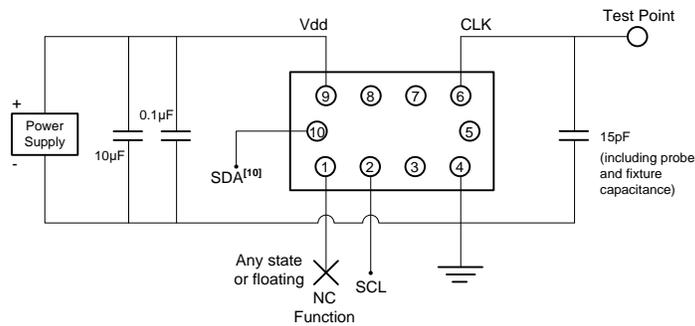
**Figure 9. LVCMOS Test Circuit (I<sup>2</sup>C Control), DCTCXO mode**
