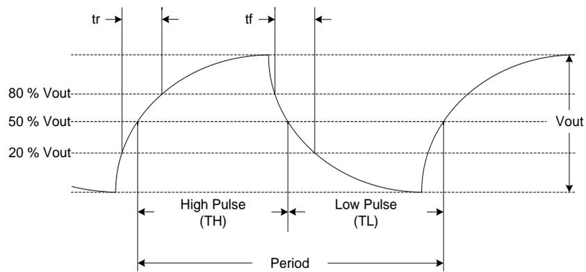
**Figure 6. Clipped Sinewave Waveform Diagram<sup>[13]</sup>**
