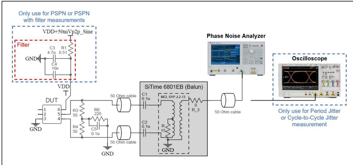
Figure 10. Test setup to measure FlexSwing Phase Noise, Period Jitter, Cycle-to-Cycle Jitter, and Power Supply-Induced Phase Noise (PSPN) with and without filter added<sup>[19]</sup>
