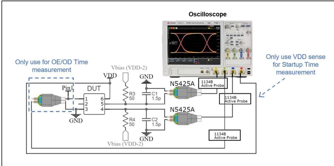
Figure 9. Test setup to measure LVPECL Waveform Characteristics, Current Consumption (with Termination 2)<sup>[17]</sup>, Output Enable/Disable Time, and Startup Time
