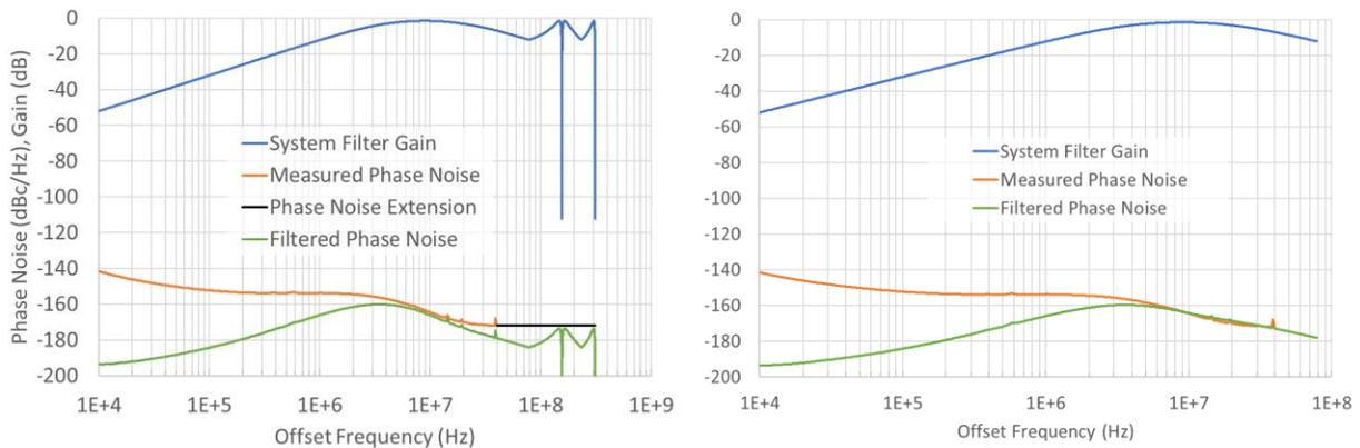
**Figure 7. Illustration of two equivalent processes to filter aliased phase noise. The left chart extends (black) the measured phase noise (orange) to the 3<sup>rd</sup> harmonic, mirrors the filter (blue) across higher Nyquist zones before deriving the filtered phase noise (green). Alternatively, the right chart aliases the extended phase noise (not shown) below the Nyquist frequency before filtering (green). Integrating either green curve produces the same phase jitter.**
