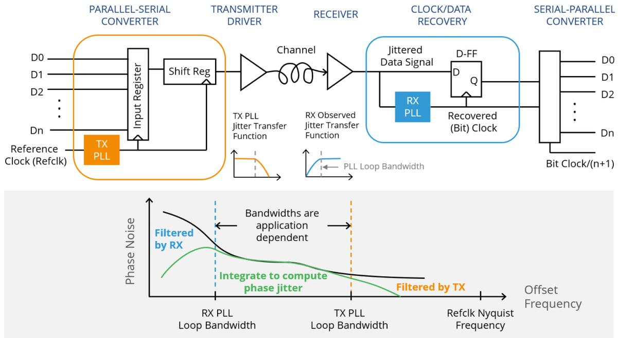
**Figure 6. A generic serial link (top) uses a transmit PLL and receive CDR to low and high pass filter, respectively, refclk phase noise. This forms a band-pass system filter (bottom) for computing phase jitter.**
