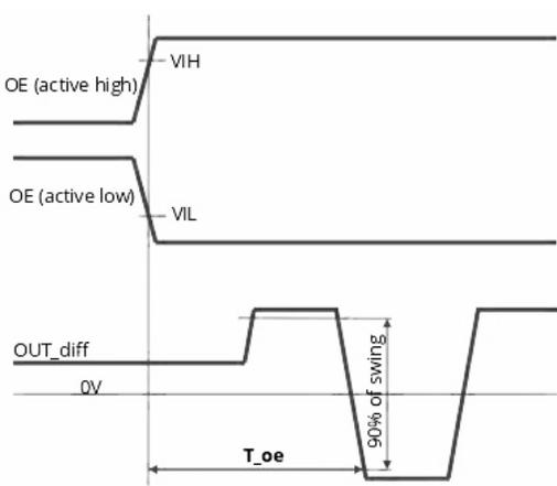
Figure 25. OE Pin Enable Timing ( $T_{oe}$ )
