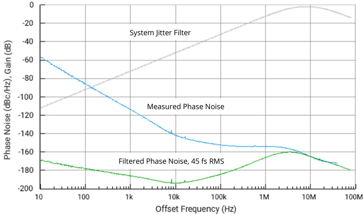
**Figure 3. Phase noise before and after filtering for SiT9501 (156.25 MHz, LVPECL, 2.5V, 25°C). The filter is applied to analyze phase noise with aliasing included up to the 3<sup>rd</sup> harmonic and features first-order filter cutoff frequencies of 4 MHz (high pass) and 16 MHz (low pass).**
