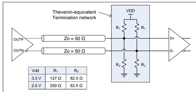
**Figure 29. LVPECL and FlexSwing DC-coupled Load Termination with Thevenin Equivalent Network<sup>[22]</sup>**
