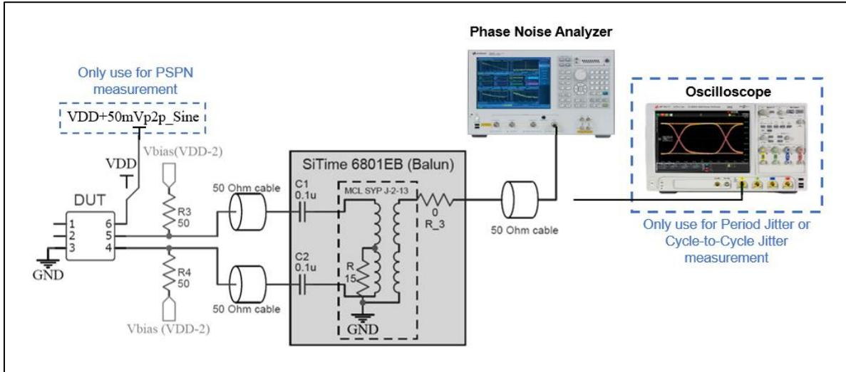
Figure 8. Test setup to measure LVPECL Phase Noise, Period Jitter, Cycle-to-Cycle Jitter, and Power Supply-Induced Phase Noise (PSPN) without filter added<sup>[16]</sup>
