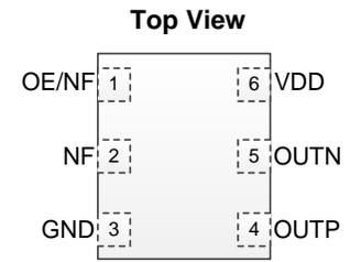
**Figure 4. Pin Assignments**
