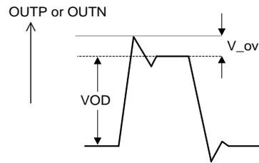
Figure 24. Overshoot Voltage ( $V_{ov}$ ) for LVDS Output
