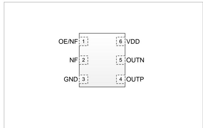
Figure 2. Pin Assignments (Top view)
