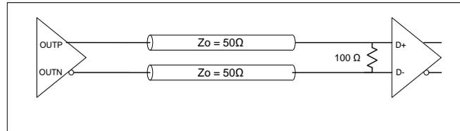
**Figure 34. LVDS DC Termination at the Load**
