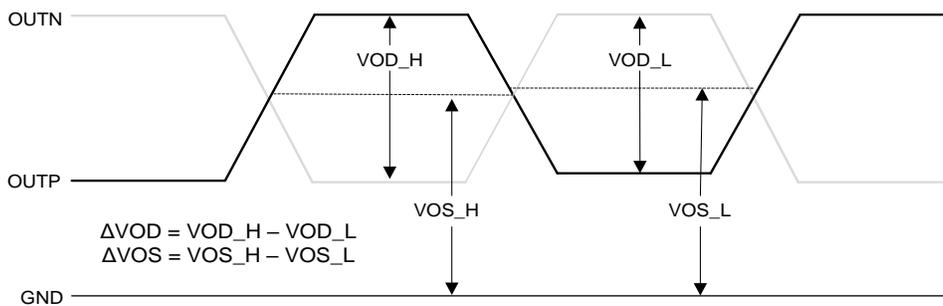
Figure 20. LVDS Voltage Levels per Differential Pin
