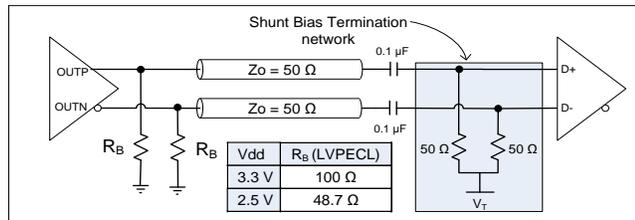
**Figure 27. Recommended LVPECL and FlexSwing<sup>[21]</sup> Termination when AC-coupled**
